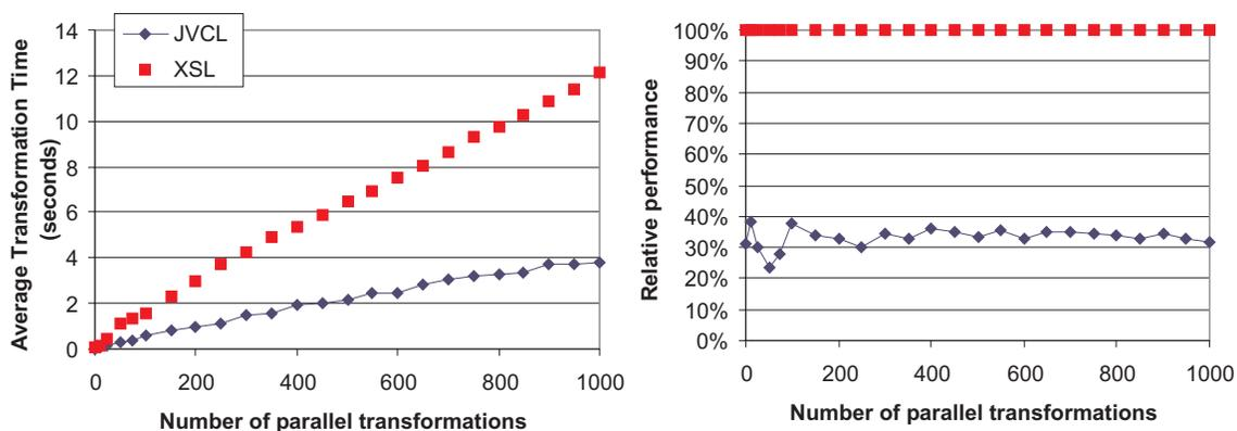
**Figure 8.2.:** *Performance of a visual mapping*
