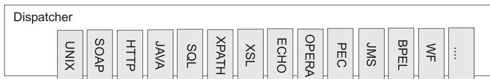
**Figure 7.7.:** *The dispatcher as a container of task execution subsystem plugins*
