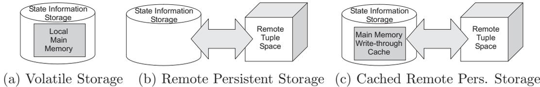
**Figure 7.4.:** *State Information Storage Implementations for the monolithic kernel*
