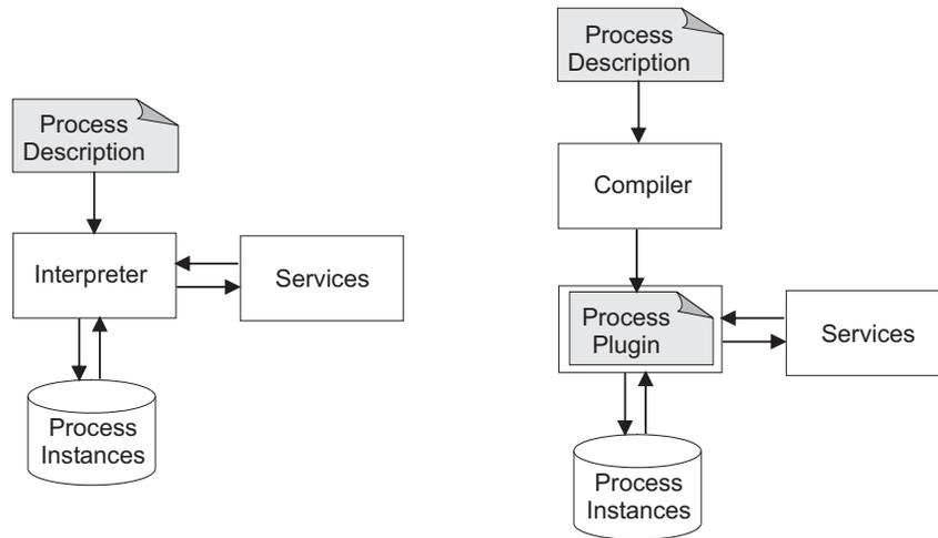
**Figure 6.1.:** *Alternative approaches to process execution.*
