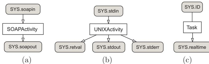
**Figure 3.11.:** *Example of system parameters and properties*
