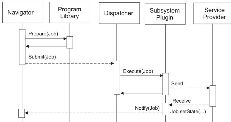
**Figure 7.11.:** *Asynchronous service invocation*
