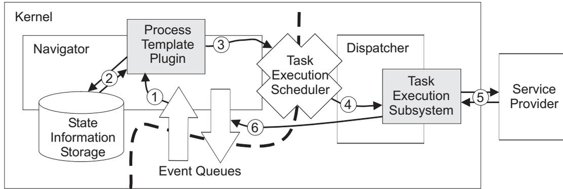
**Figure 7.5.:** *Main Process Execution Loop*
