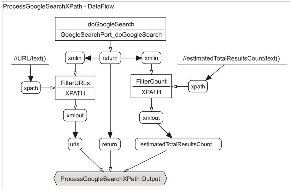
**Figure 4.7.:** *Example of XML Processing with the JVCL and X-Path.*
