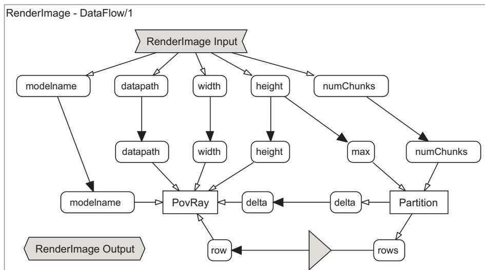
**Figure 4.14.:** Data flow view of the first part of the `RenderImage` process
