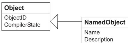
**Figure 5.8.:** *Abstract Elements: Object and Named Object. All OML Elements inherit their basic attributes from these two elements.*
