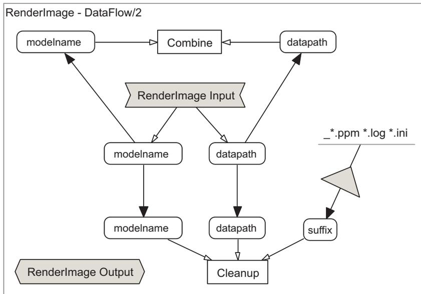
**Figure 4.15.:** *Data flow view of the second part of the `RenderImage` process*
