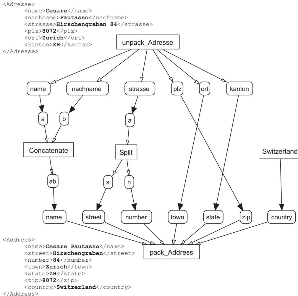
**Figure 4.11.:** Visual mapping between two XML complex types
