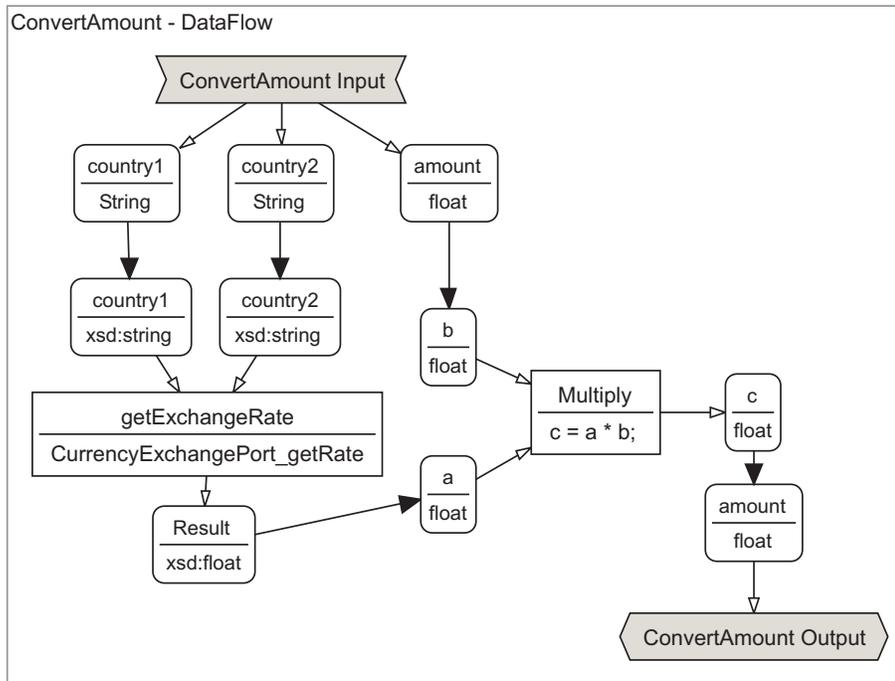
**Figure 4.5.:** *Data flow view of the ConvertAmount process*
