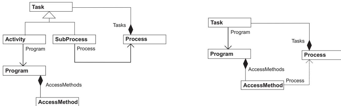
**Figure 5.15.:** *Simplified Task Model. Comparison between the original OML model (left), which includes the Activity and SubProcess elements, with the simplified model (right), where there are only Tasks.*
