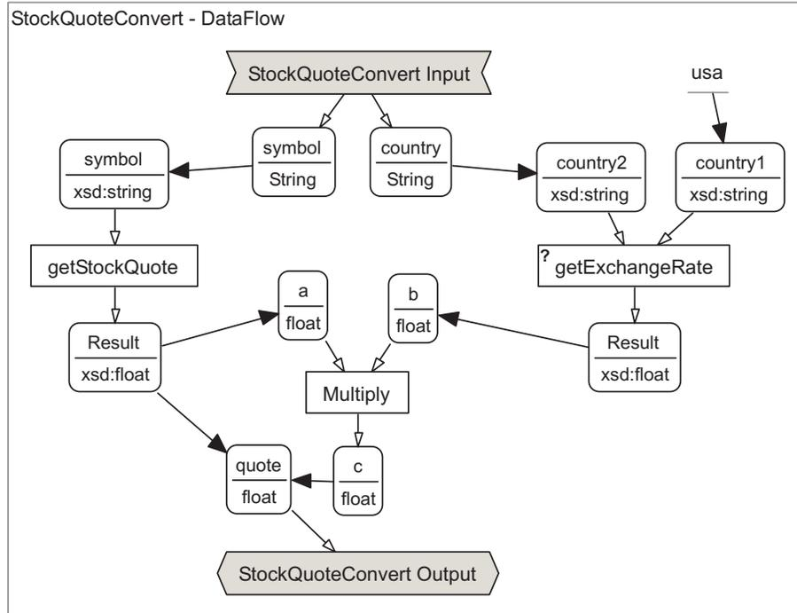
Figure 4.6.: Data flow view of the `StockQuoteConvert` process
