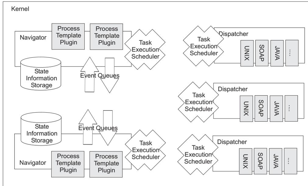
**Figure 7.14.:** *Architecture of a Peer to Peer Process Execution Kernel*
