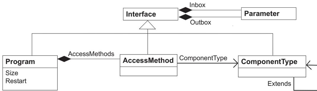
Figure 5.14.: Structure of the Program and Component type library.
