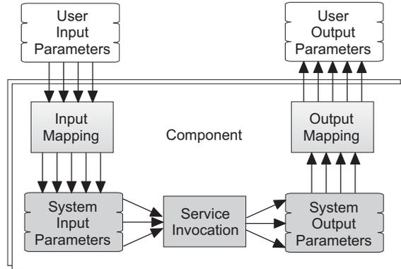
Figure 4.2.: *Data flow mapping inside a component*
