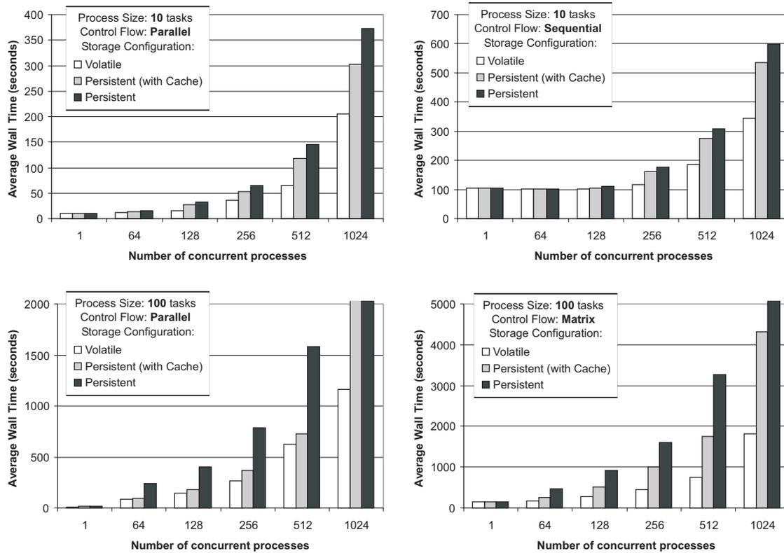
**Figure 8.3.:** *Performance degradation of a centralized process support system under increasingly large workloads*
