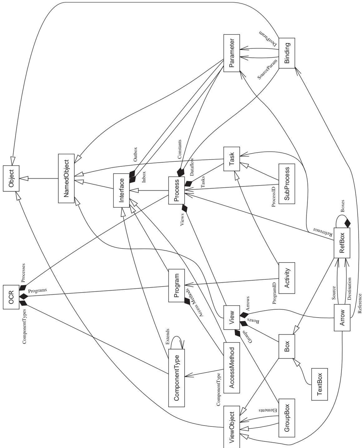
**Figure 5.6.:** Complete UML class diagram of the OML elements. For completeness, we include also this UML class diagram with all relationships between all elements of an OML document.
