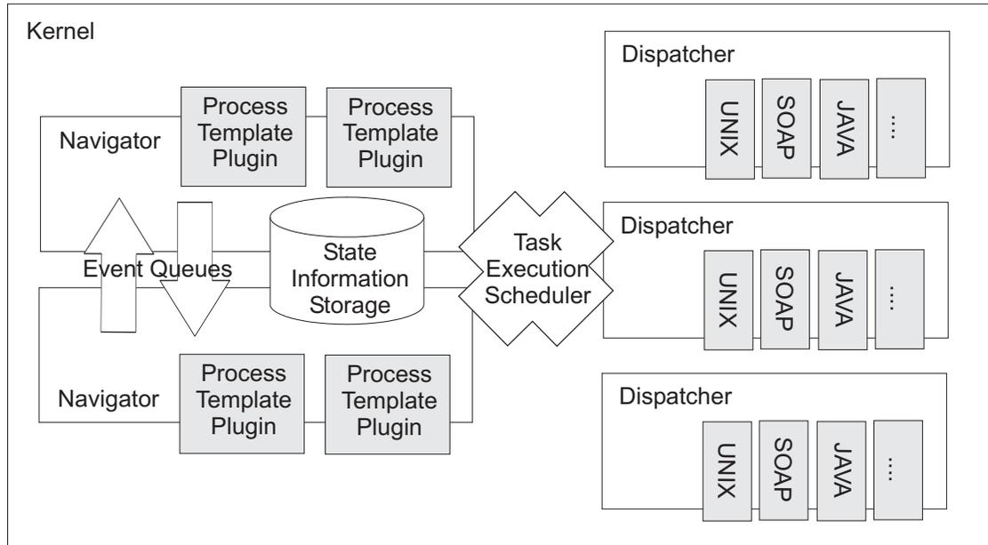
**Figure 7.6.:** *Architecture of a Distributed Kernel*
