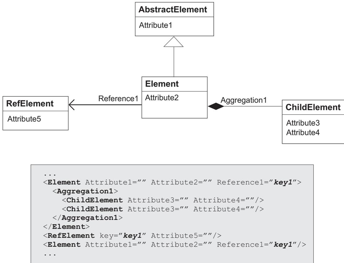
**Figure 5.1.:** Mapping UML to an XML document. Example of the relationship between the syntax of a UML class diagram (above) and the corresponding XML document structure (below) as it is defined in our Meta-Meta model. For clarity, the values of most attributes have been omitted.
