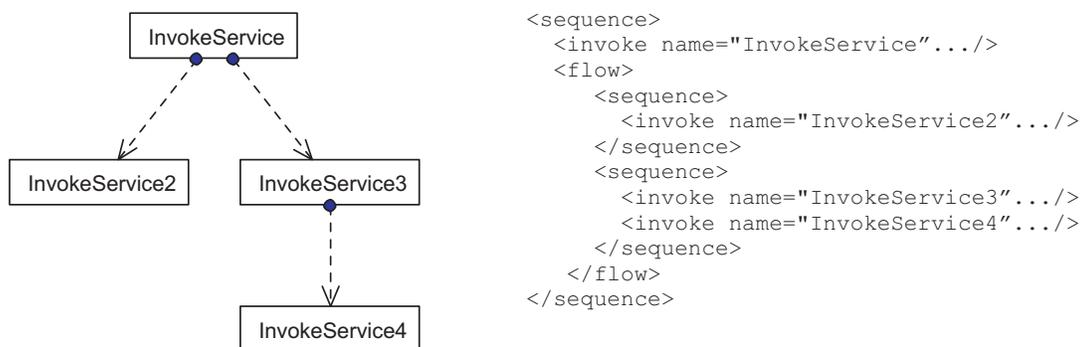
**Figure 6.5.:** A process invoking multiple Web services shown both in JVCL and in BPEL. There is a clear correspondence between the block-based structure of the BPEL representation and the control flow graph of the JVCL.
