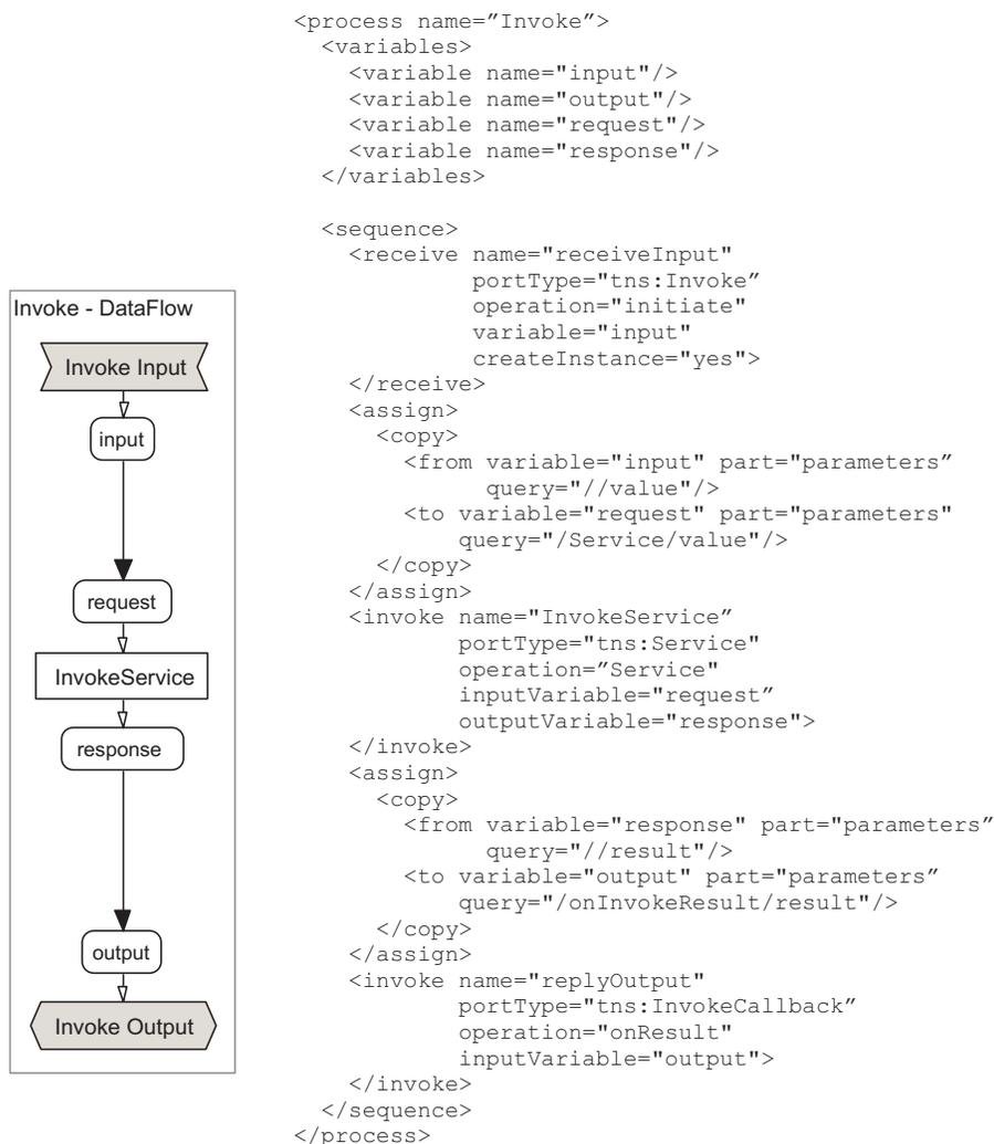
**Figure 6.4.:** A process with a single Web service invocation represented both in JVCL and in BPEL. The corresponding parts of the process are shown side by side.
