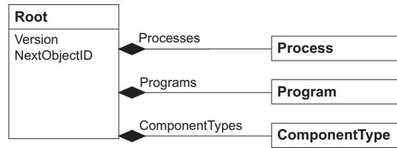
**Figure 5.7.:** *Basic structure of an OML document. An OML document is composed of Processes, Programs and Component Type definitions.*
