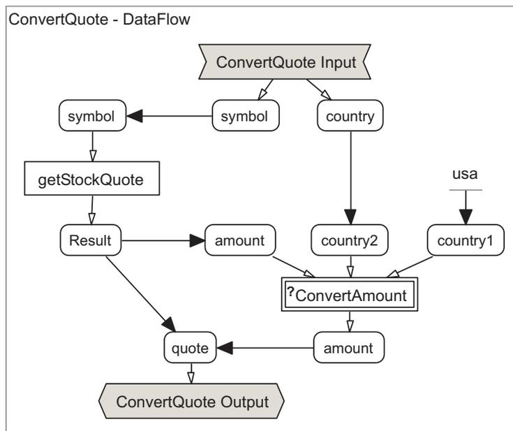
**Figure 4.4.:** *Data flow view of the ConvertQuote process*
