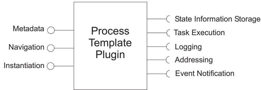
**Figure 6.9.:** *Process Template Plugin Interface*
