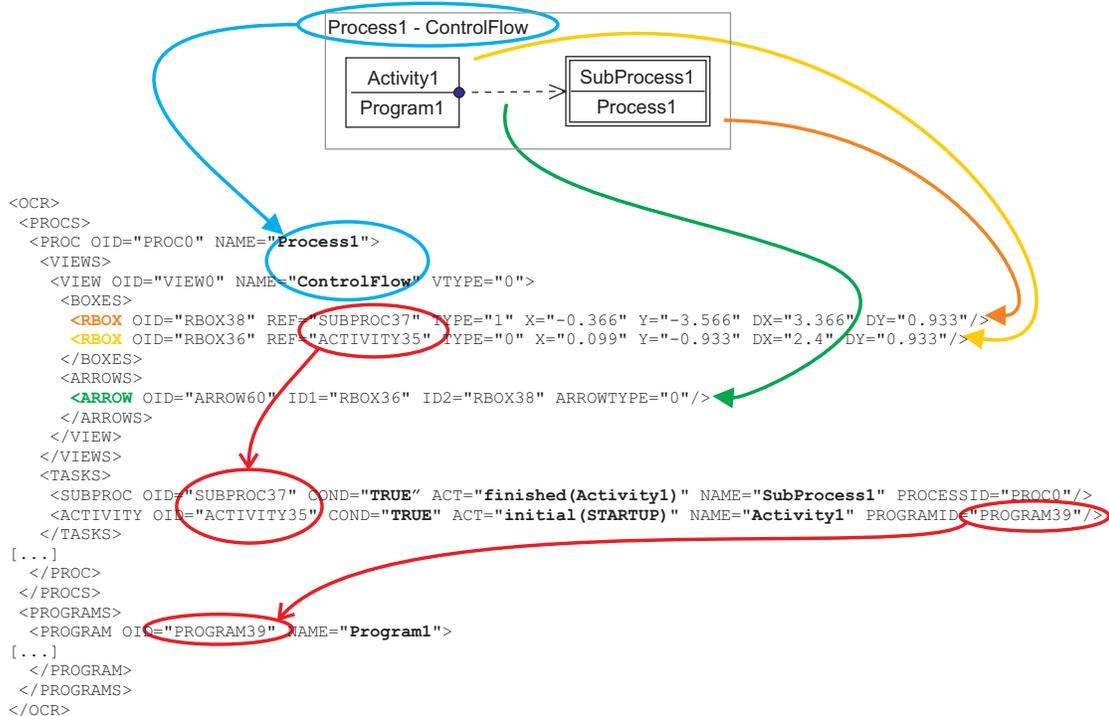
**Figure 5.13.:** Example on how a JVCL control flow view is stored in the underlying OML model. Each visual object (the Process, the Activity, the Sub-Process and the Control flow dependency between them) corresponds to an element of the OML document. The text shown inside the boxes is stored in the corresponding document elements. The RefBox elements are linked to the referenced task elements, as it is possible to display the same task in multiple views.
