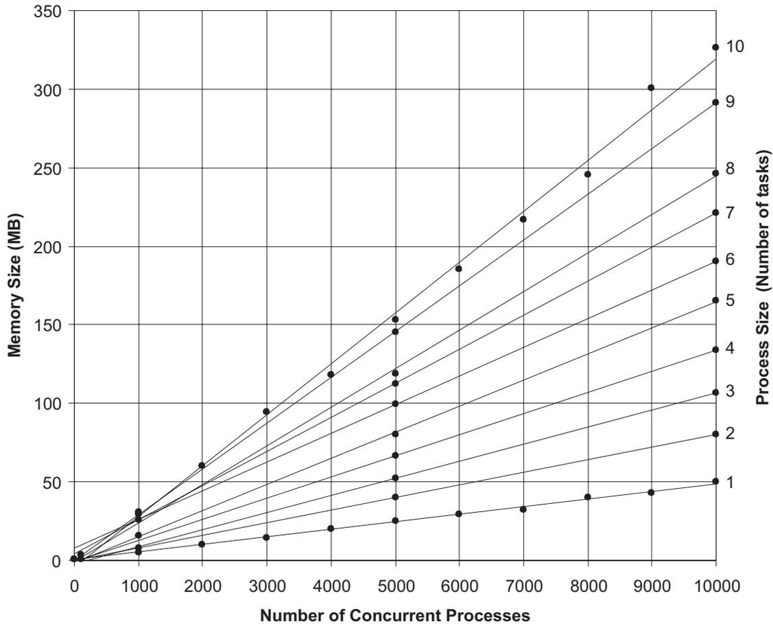
Figure 8.6.: *Memory requirements for process instantiation*
