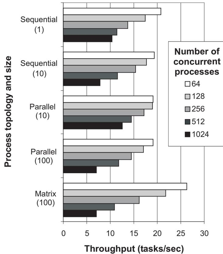
**Figure 8.4.:** *Throughput degradation of a centralized process support system under increasingly large workloads*
