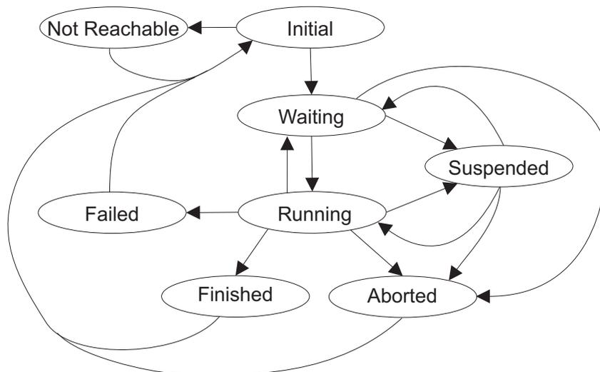
**Figure 6.7.:** *Simplified state diagram of a task instance as it is seen by the user*
