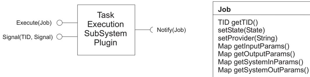
**Figure 7.8.:** *Interface definition of the task execution subsystem*
