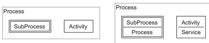
**Figure 3.1.:** *Syntax definition for the Activity and the SubProcess*
