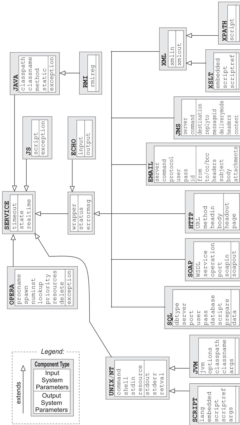
Figure 4.3.: Summary of the System Parameters of some the component types modeled in this chapter
