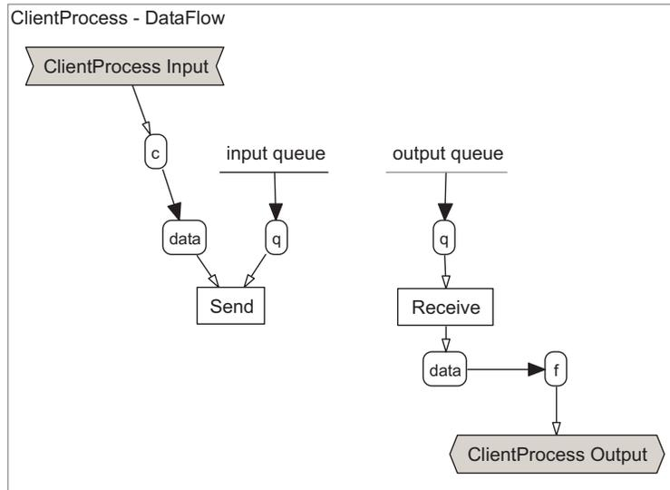
**Figure 4.16.:** *Data flow view of the ClientProcess*
